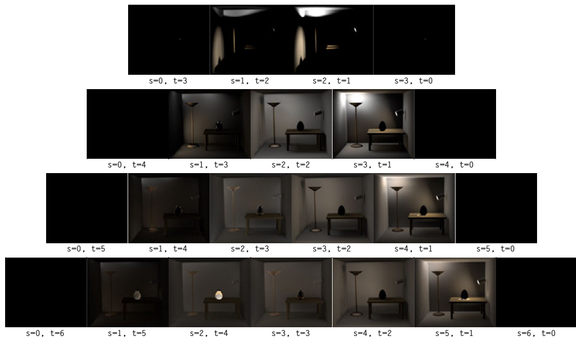
(b) The same sampling strategies, but now weighted using multiple importance sampling—effectively “turning off” each strategy where it does not perform well. The final result is computed by summing all of these images.
