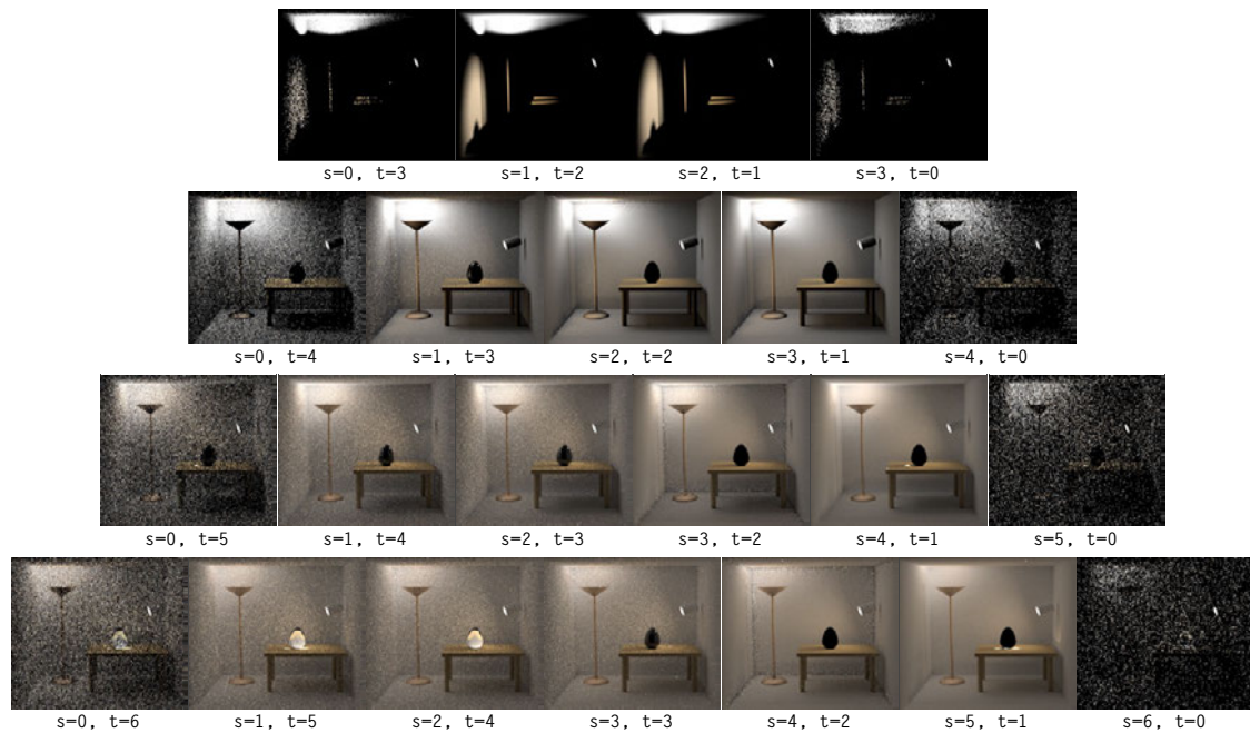
(a) The individual sampling strategies that comprise BDPT, but without multiple importance sampling. s denotes the number of steps taken from the emitters, and t denotes the number of steps from the sensor. Note how almost every strategy has deficiencies of some kind
