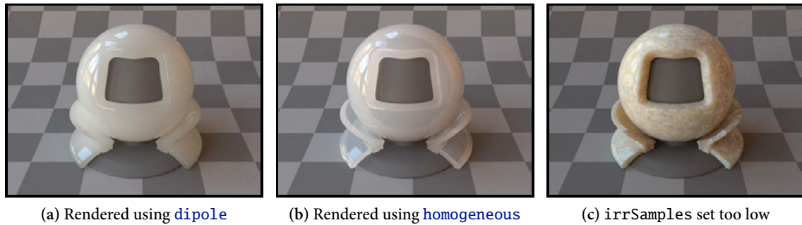
Figure 19: Two problem cases that may occur when rendering with the dipole : (a)-(b): These two renderings show a glass ball filled with diluted milk rendered using diffusion theory and radiative transport, respectively. The former produces an incorrect result, since the assumption of many scattering events breaks down. (c): When the number of irradiance samples is too low when rendering with the dipole model, the resulting noise becomes visible as “blotchy” artifacts in the rendering.
